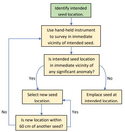
Figure 1: Anomaly Avoidance During Seed Emplacement
