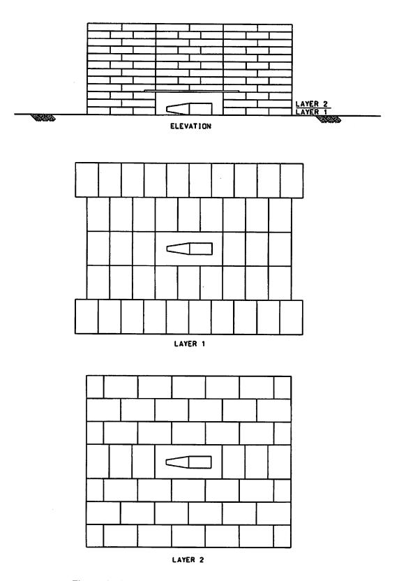
Figure 6 - Interlocking Alternate Layers of Sandbags
