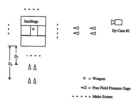
Figure 1 – Site Layout for Tests of Sandbag Enclosures
