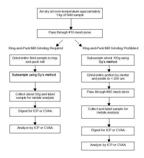
**If Ring and Puck Mill grinding is required,** then proceed with the grinding procedure listed in this SOP for explosives. The metallic components from the Ring and Puck Mill may introduce chromium and iron into the sample.
